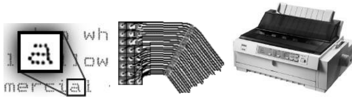
Figure 2.15: Dot Matrix Pins
